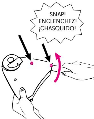
Swing the legs outward until the single button snaps into its notch, as shown. CHECK that the legs are properly attached by twisting them in the housings.
